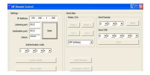
10. On connection, press the Parameter / HW-ID. A new window will open. Enter 0x0606 in Address field and press read button. Confirm that Data [8-bit] reads 0x00 and Status say EEProm read Successful! (see picture below left). Now enter 0x01 in Data [8-bit] field and press Write button. That should write the new setting on to EEProm. To confirm the setting has been written press Read again and that should show 0x01 in the Data field.
